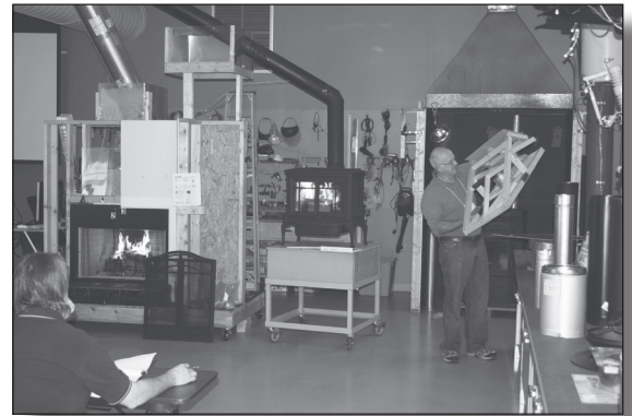
A fireplace and wood-burning stove operate with real-time temperature recording so you can see how varying conditions can affect temperatures inside the appliances and on the exteriors of their chimneys or chimney connectors. Mockups of roof structures illustrate how and why chimneys are installed improperly and cause fires.
